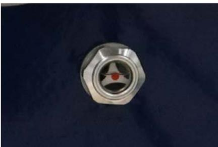
If the oil sight glass is filled or the surface is visible in the top of the oil glass the oil level is OK.
