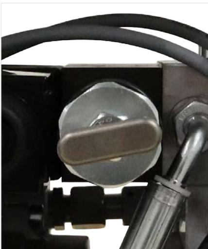
Adjustment is done using the pendant and the adjustment screw (see picture).
