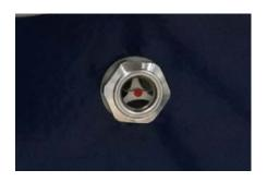
If the oil sight glass is filled or the surface is visible in the top of the oil glass the oil level is OK. If not, the oil level has to be checked with the oil stick in the filling plug - The surface must be approx. 30 mm below the top of the tank.
